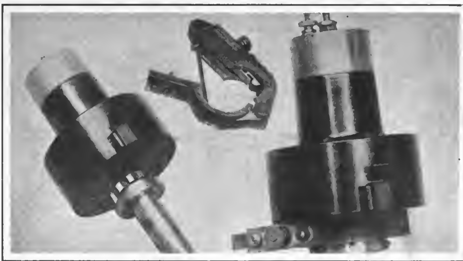
Fig. 1—Pittsfield distributor complete and with the breaker mechanism removed. The method by which the breaker box comes off is obvious. The coil is contained in the upper part of the body which is stationary, only the breaker moving to give advance
